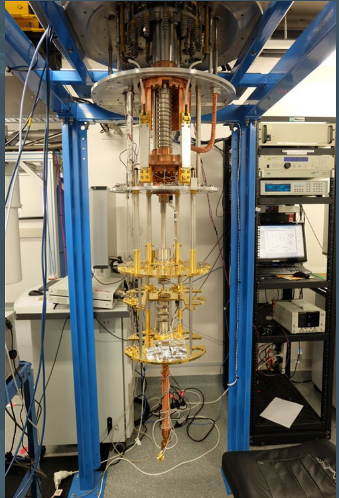
The dilution refrigerator used to cool ORGAN down to cryogenic temperatures
