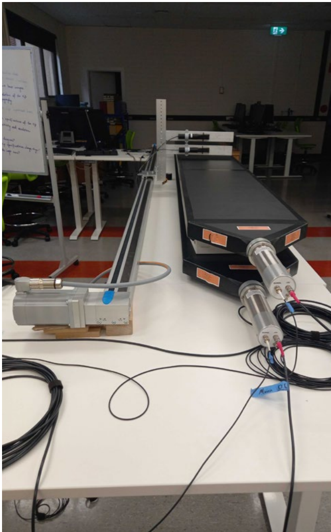
Two of the muon detectors being tested with a calibration stage at UoM.
