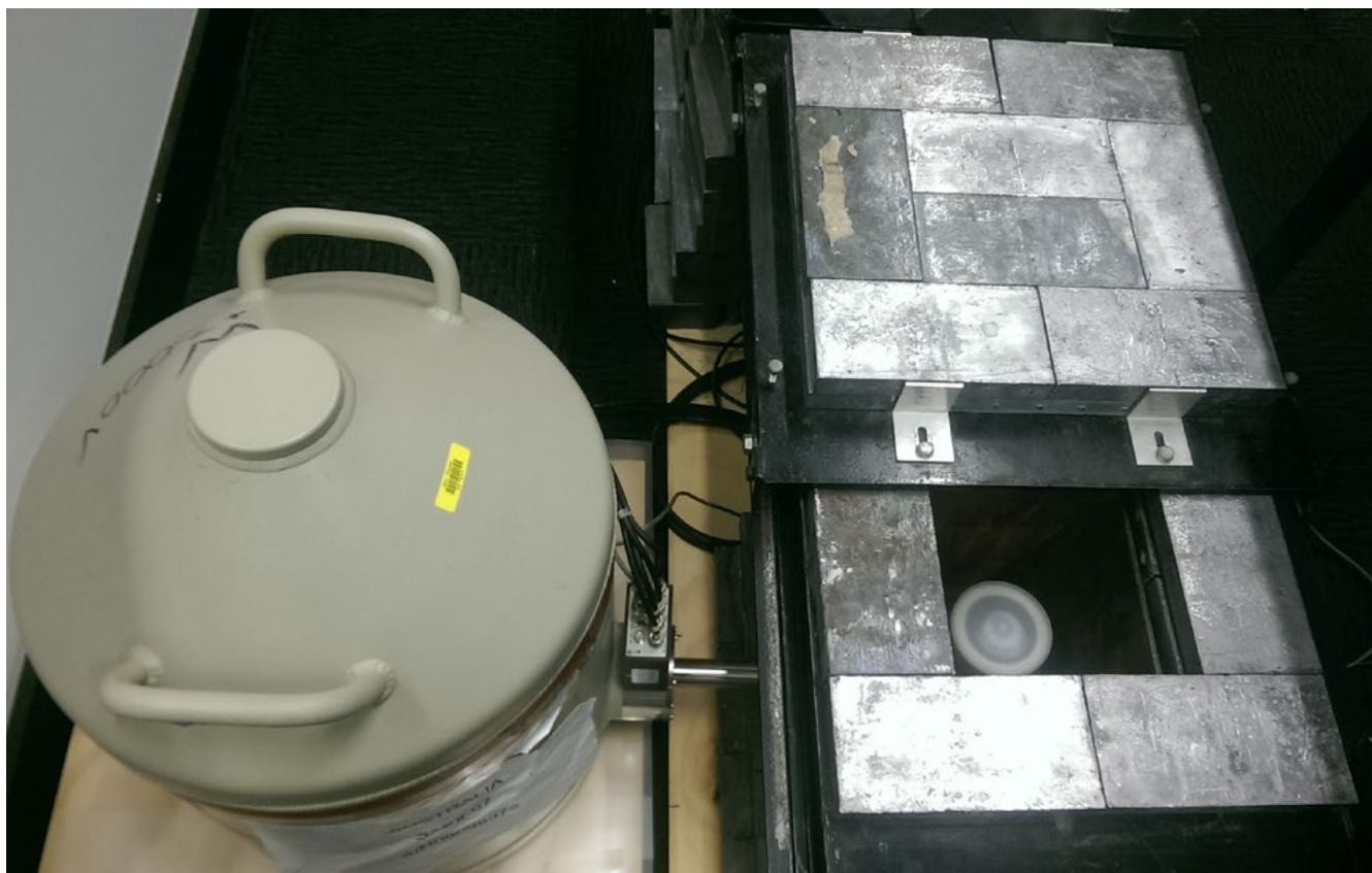
Newly installed germanium detector at ANU.
