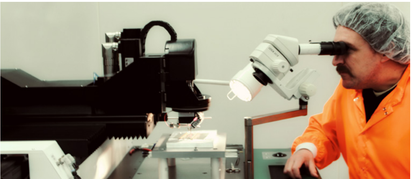
ITK module construction at the UoM silicone clean room.
