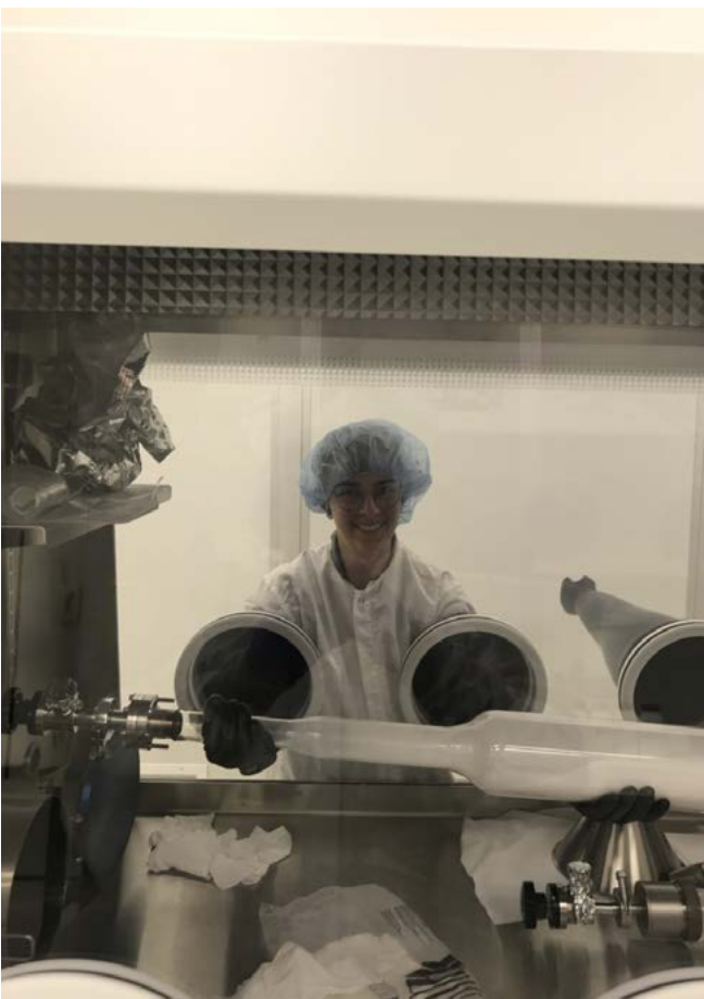
The NaI-33 crystal prior to Teflon wrapping.
