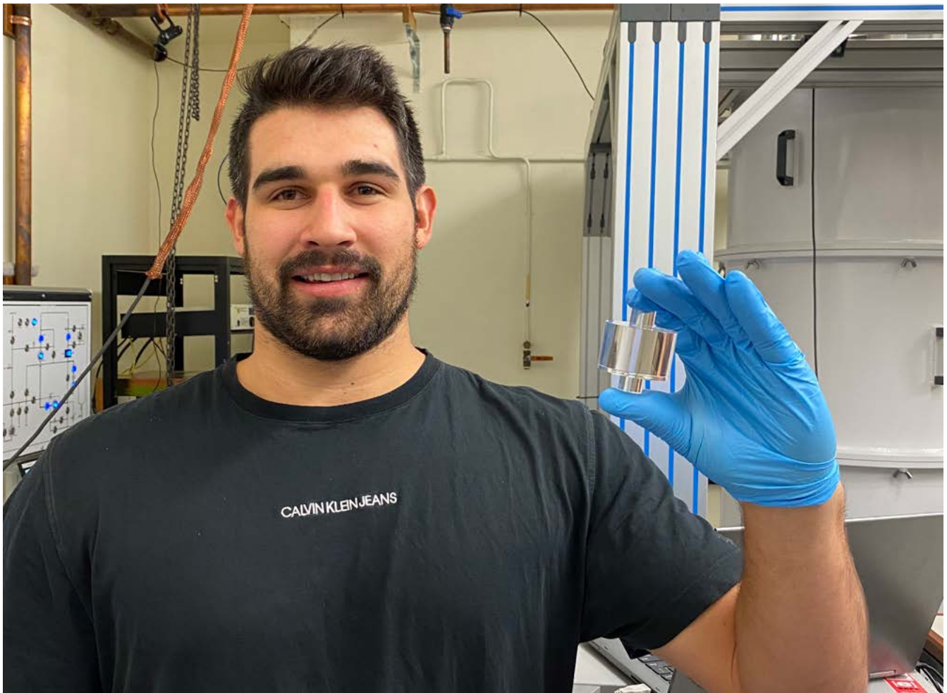
Aaron Quiskamp, holding a sapphire resonator and standing in front of a mK BlueFors dilution fridge, undergoing low temperature measurement of microwave cavities under large magnetic fields. His new DBAS resonator will be manufactured from sapphire and will sit inside a 14 T magnetic field to search for axions with the ORGAN dark matter detector.
